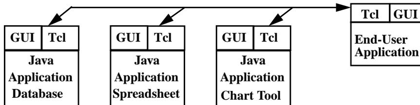
Figure 1. Tcl can be used to give a suite of Java applications a common interface for extending the applications and for end-user customization. This notion is similar to how Microsoft extends it’s Office application suite with VBA.
