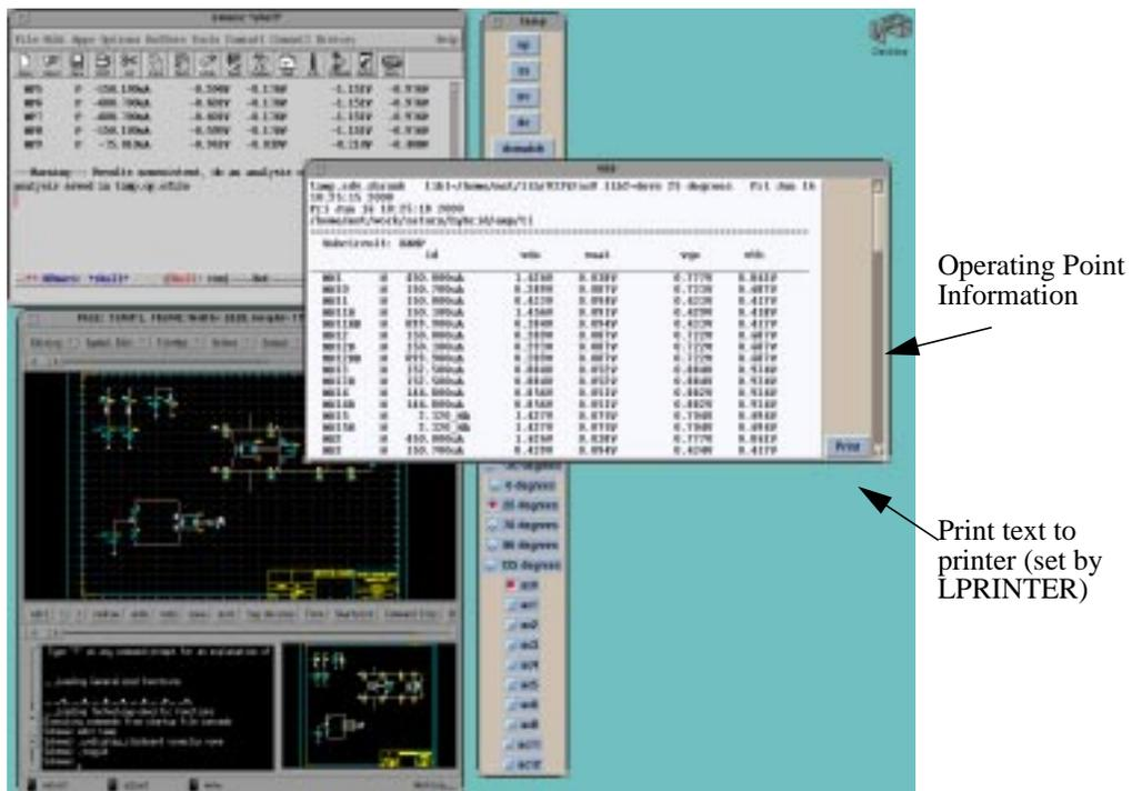
Figure 4: Screen Shot after performing Operating Point Analysis
