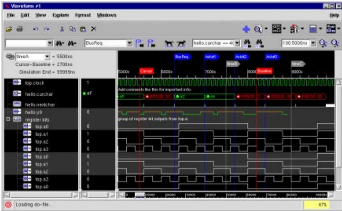
**Figure 1: Main window of the SignalVision waveform plotting tool. The tool is a mixture of custom-built widgets, BLT widgets, and [incr Tcl/Tk] mega-widgets, all stitched together with Tcl code.**
